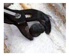
At this temperature the ball will move through the foam but not cause a flame. If it is too hot you will end up with a very large chasing.
